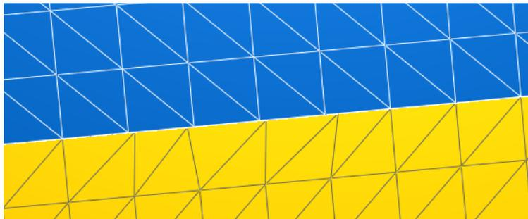
Fig 1.5: The center nodes of both grids are not in contact with each other. This is a grid error as the current cannot pass such a line. Of course this is an unsuitable method for modeling small physically existing apertures! In such a case the typical size of patches close to a long narrow opening should not get larger than the width of that opening or aperture respectively.
