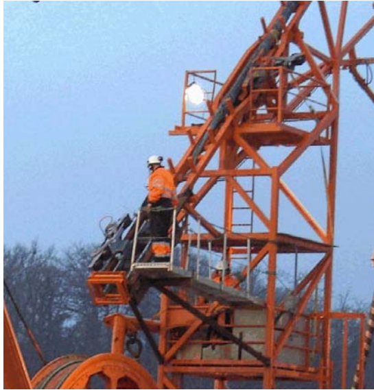
Figure 11. An extension was built on the “gooseneck” where the vespa was built-in.
