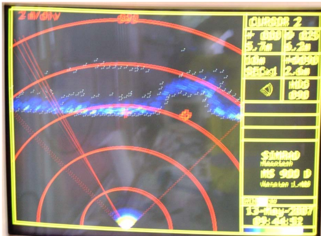
Figure 21. Plot of the profile above the trench. The blue is the surface of the seabed and the red circles every second meter from the profiler in the centre. The profiler is not directly over the trench.
