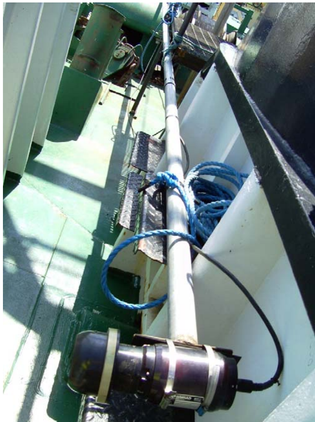
Figure 20. The profiler seen is attached to a steel tube, and is fastened at the bow, one meter below sea level.
