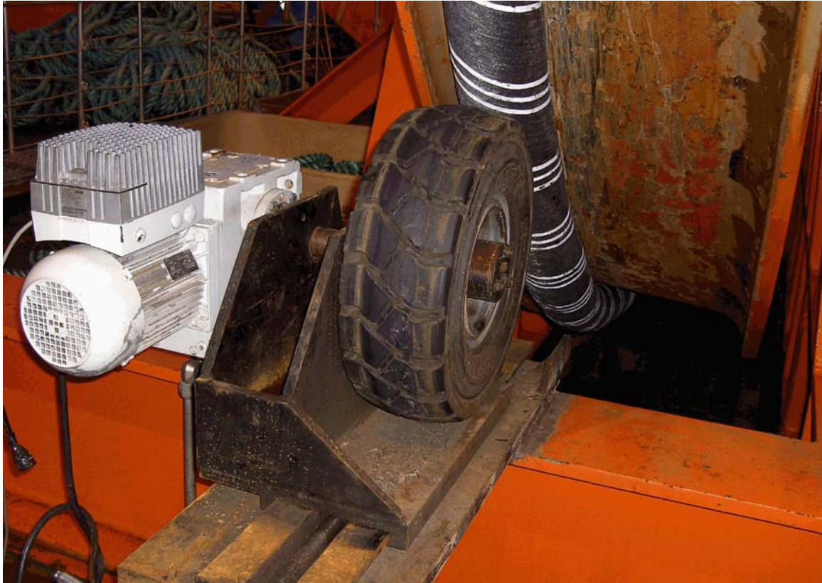
Figure 10. The motor installed with the wheel pressing onto the cable at the capstan.
