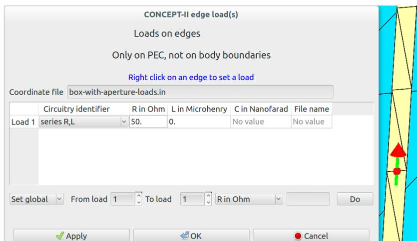
Fig 5: Window for setting edge loads
