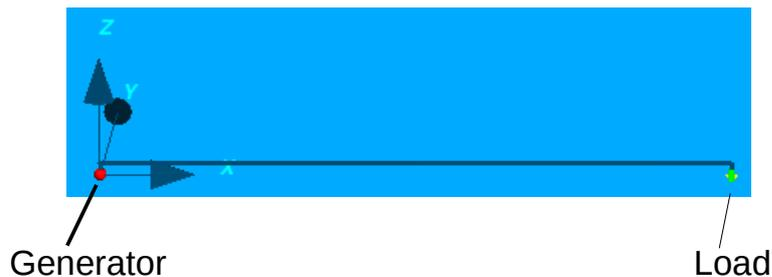
Fig 5.4: Single-wire transmission line over an ideal ground excited by a voltage jump
